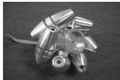
Figure 8.1: Mecanum wheel designs with rollers at 45°
