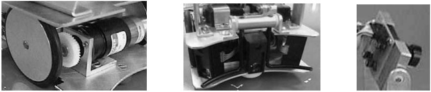
Figure 18.3: Sensors: shaft encoder, infrared sensors, digital camera
