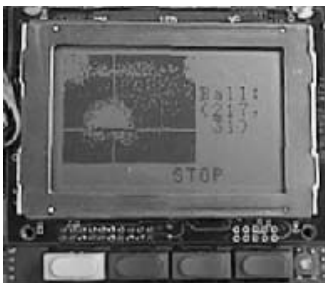
Figure 18.6: LCD output after ball detection
